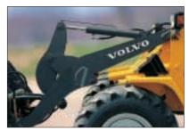
Z-bar loader linkage with high lifting capacity and breakout force.
